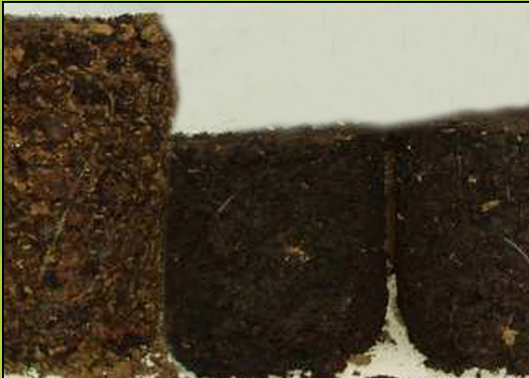
Stable RHP coir (left) & unstable decomposed coir (right).
